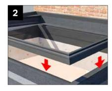
Position PVCu welded base frame and align with internal kerb face.
