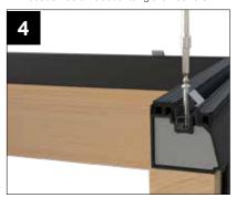
Firstly check that all aluminium spacer sleeves are in place in the fixing holes Ensure you use all the clips provided. Position clips (FRICB001M) into location holes and fix using the provided (FRFC008-100) 100mm long screw.
